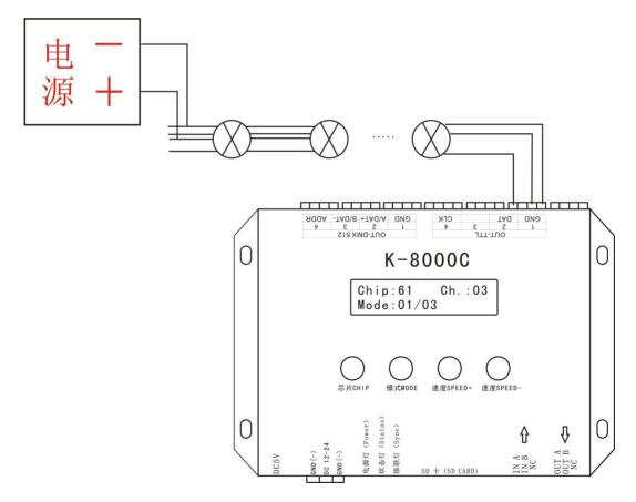
1.Like the above diagram, wired the line and start the controller, press "CHIP" and "MODE" at the same time switch to coding mode, adjust to Chip: 61 that is UCS512A or B coding mode, as below:
