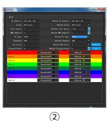
The left column is the original data in the controller, and the right column is the modified data.
